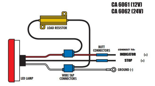
Insert Wires, squeeze with pliers to snap, splice tap shut - Do not cut your vehicle Wires
